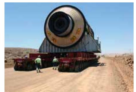
Transport of giant grinding mill along services corridor
